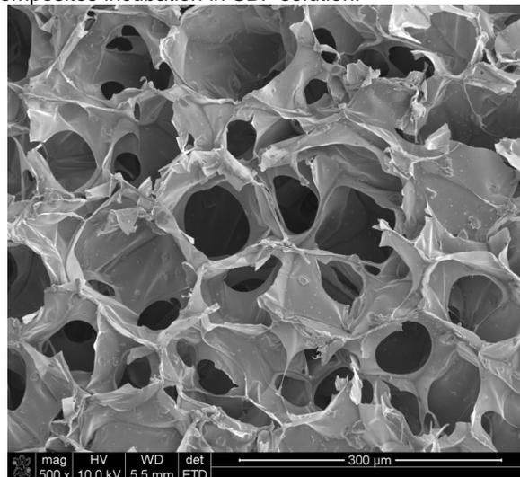
FIG. 1. SEM image of P5Zn1gCH\_1:1 composite microstructure.
