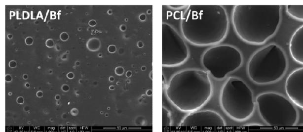
FIG. 2. Microstructure of drug-modified membrane materials (biofuroxsim)
