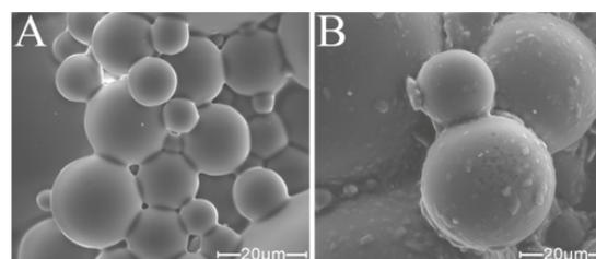
FIG. 2. SEM micrographs of PMMA (A) and PMMA/PEG/AA system 9:1 (B).
