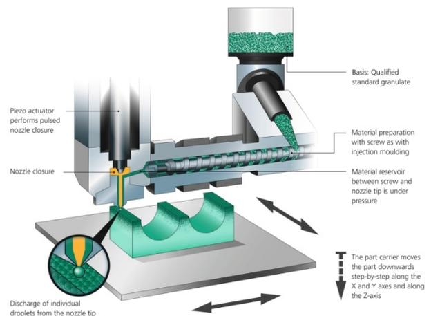
FIG. 2. The APF process principle in detail.
