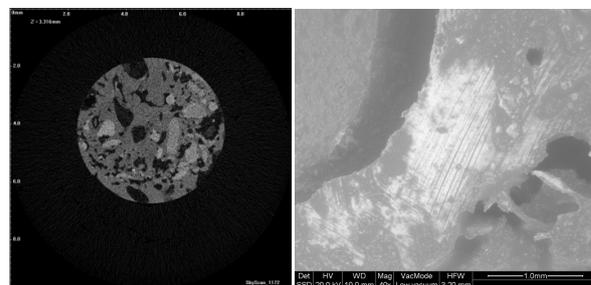
FIG. 2. MicroCT cross section of 90% -TCP-10% geopolymer, implanted in New Zealand femur and the relevant histological picture.
