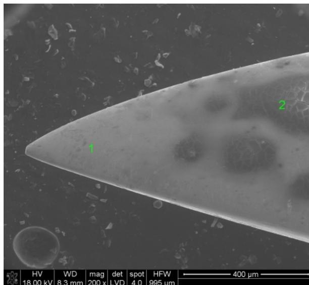
FIG. 2 SEM of Kirschner wire after one month of implantation.
