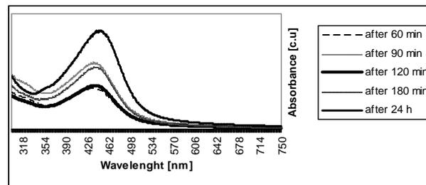
FIG. 1. UV-vis spectra of silver suspension from Tchibo coffee-water at room temperature depending on synthesis time.
