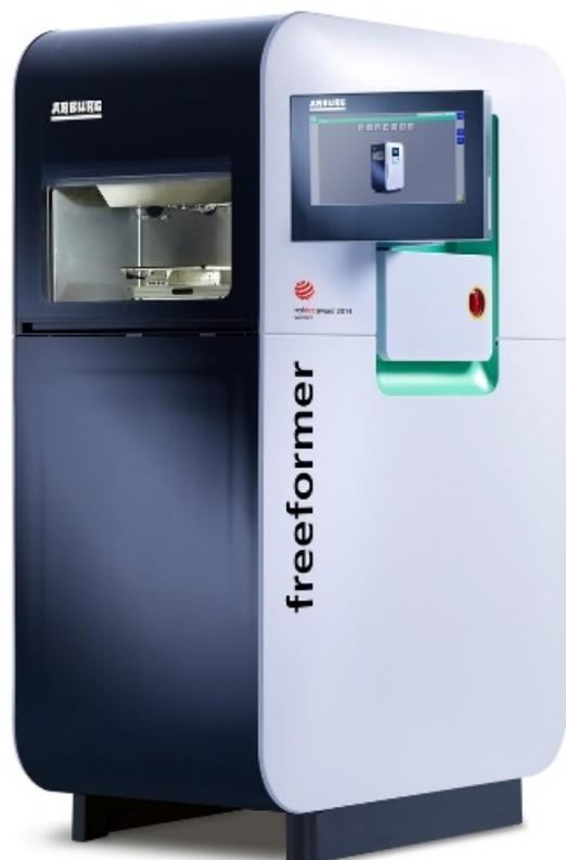
FIG. 3. Freeformer: Open production system for the APF process.
