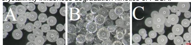
FIG. 1. Photographs of microparticles: A – reference MS1, B – MS2 – water phase modified with NaCl, C – MS3 – oil phase modified with PEG400. Scale bar 100  $\mu\text{m}$ .
