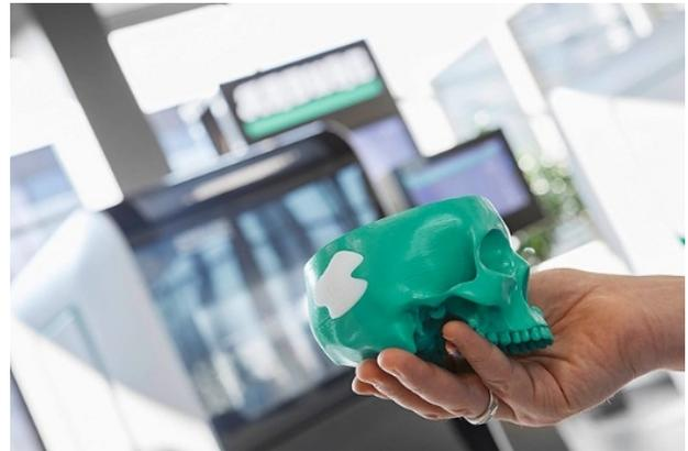
FIG. 1. Individually adapted implant for cranial bones was produced in the APF process using medical grade PLA granulate (Resomer).
