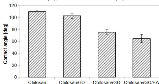
FIG. 2. Effect of nanofillers and HAP on contact angle.
