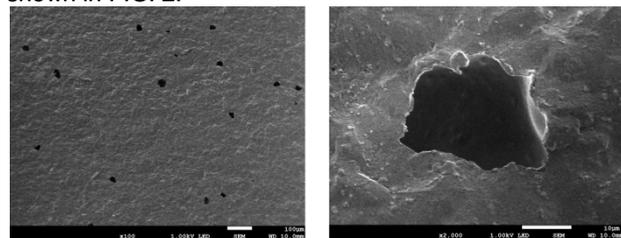
FIG. 2. Topography of bone cement and sample pore.
