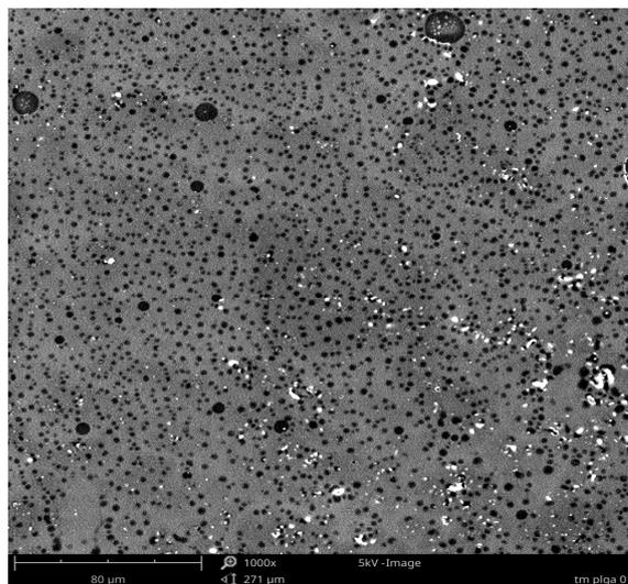
FIG. 1. SEM image of hybrid oxide-ceramic coatings formed on Ti-15Mo alloy surface. Magnification: x1000.
