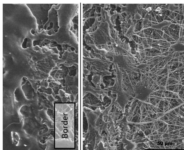
FIG. 2. Effect of UV and O<sub>3</sub> on the PLA fibers after 24 h exposition.
