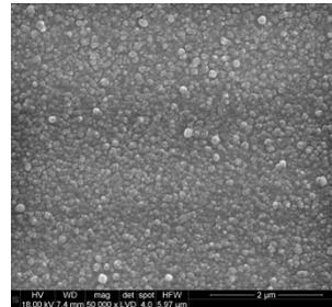
FIG. 1. SEM image for series 1C (mag. 50 000 x).
