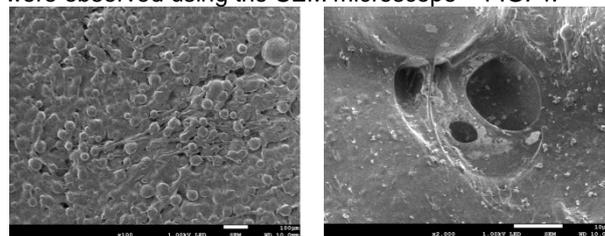
FIG. 4. Topography of bone cement after corrosion test.
