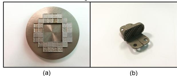
FIG. 1. (a) Samples produced with different manufacturing parameters; (b) Spinal disc replacement.
