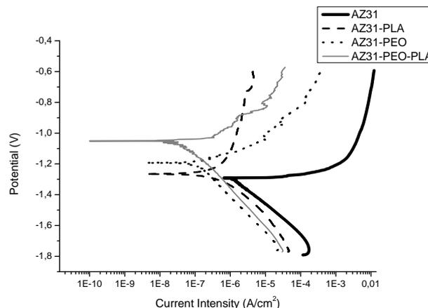
FIG. 1. Potentiodynamic polarization curves of the samples exposed to Hanks solution.
