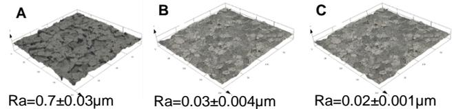
FIG. 2. 3D images of Ti surface after treatment using 5%HF (A), pyrolytic carbon (B), Ar ion beam (C), and values of roughness (Ra).
